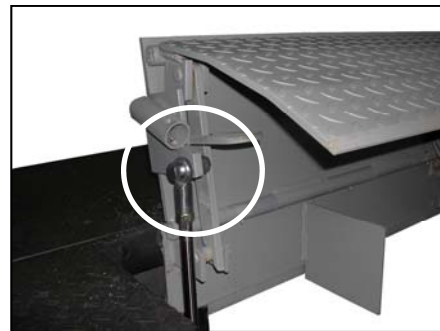
Cylinder connection to ramp plate
